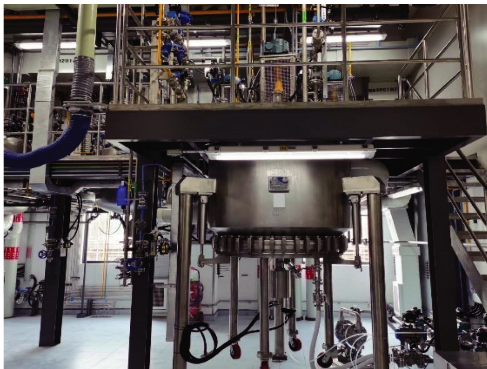
This 1,000 L peptide synthesizer is at WuXi STA's Changzhou, China site.
